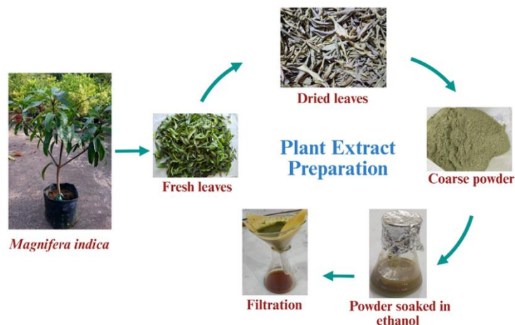
Fig. 1. Different steps in plant extract preparation for nanoparticles synthesis.
