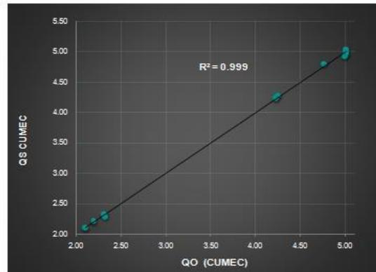
**Fig.13.** Relationship between observed and simulated Seepage at the different reservoir levels.
