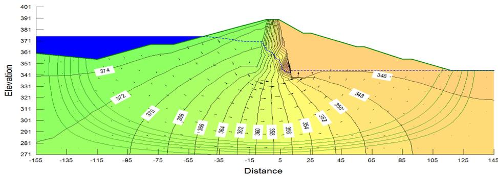
Fig.11. Simulated Flow-net Profile at EL 375 m.
