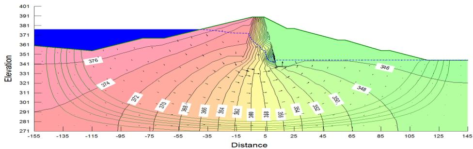
Fig.9. Simulated Flow-net Profile at EL 377 m.
