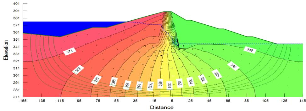
Fig.10. Simulated Flow-net Profile at EL 376 m.
