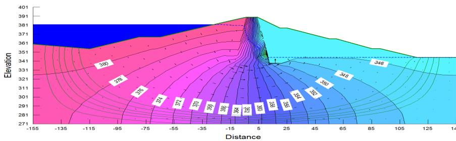
**Fig.4.** Simulated Flow-net Profile at EL 382 m.
