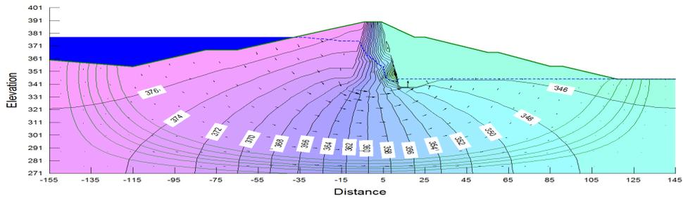
Fig.8. Simulated Flow-net Profile at EL 378 m.
