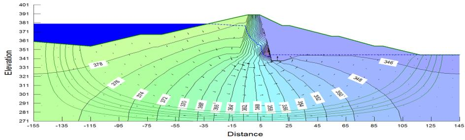
Fig.6. Simulated Flow-net Profile at EL 380 m.
