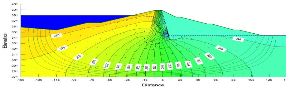
**Fig.5.** Simulated Flow-net Profile at EL 381 m.
