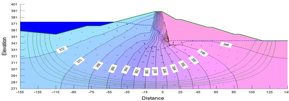
Fig.12. Simulated Flow-net Profile at EL 374 m.
