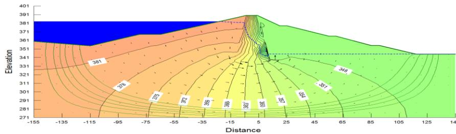
**Fig.3.** Simulated Flow-net Profile at EL 383 m.
