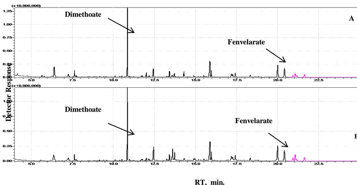
**Fig. 2.** Chromatogram Showing the Effect of Addition of C18 Cartridge Used as a Sorbent for Cleaning Extract of Cucumber Spiked Sample, A: Without C18, B: With C18.
