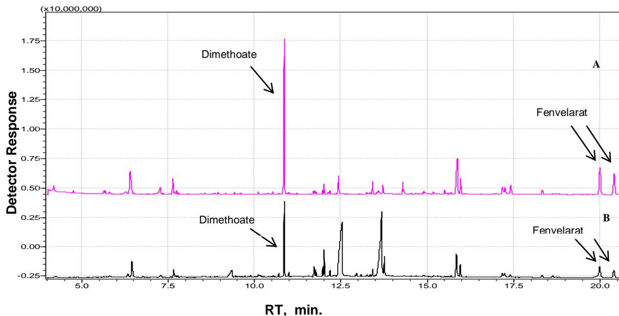
**Fig. 3.** GC-MS Chromatogram of Cucumber Extract: A: Extract spiked with 1 ppm pesticides mixture. Extract was cleaned via c-SPE procedure using 400 mg PSA, 400mg charcoal, B: extract spiked with 1 ppm pesticides mixture. Extract was cleaned via d-SPE using 100 mg charcoal, 400 mg PSA, eluted with Acetonitrile :Toluene (3:1), Reconstitute in acetone: hexane(1:9).Chromatogram were made in the same scale. Injected volume: 1  $\mu$ l for c-SPE and d-SPE.
