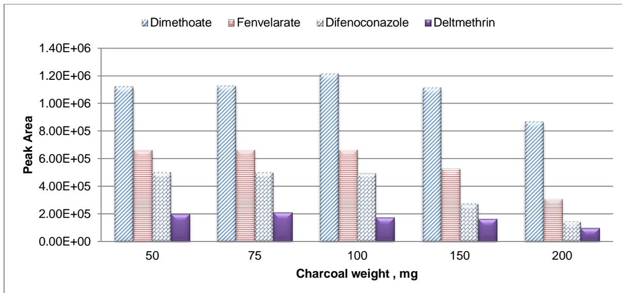
Fig. 1. Effect of Charcoal Weight Used in d-SPE on the Cleanup of 1 ppm Spiked Cucumber Samples.
