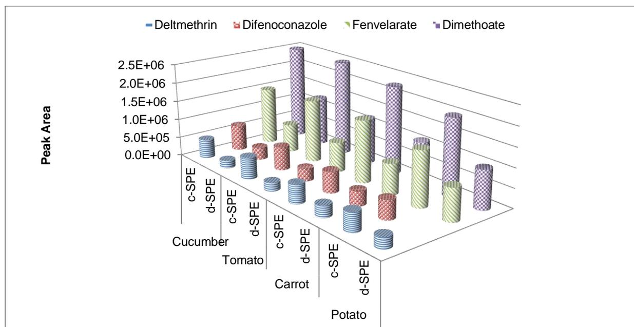
**Fig. 4.** Sample Preparation Efficiency Using d-SPE and c-SPE for Selected Pesticides in Vegetables Samples.
