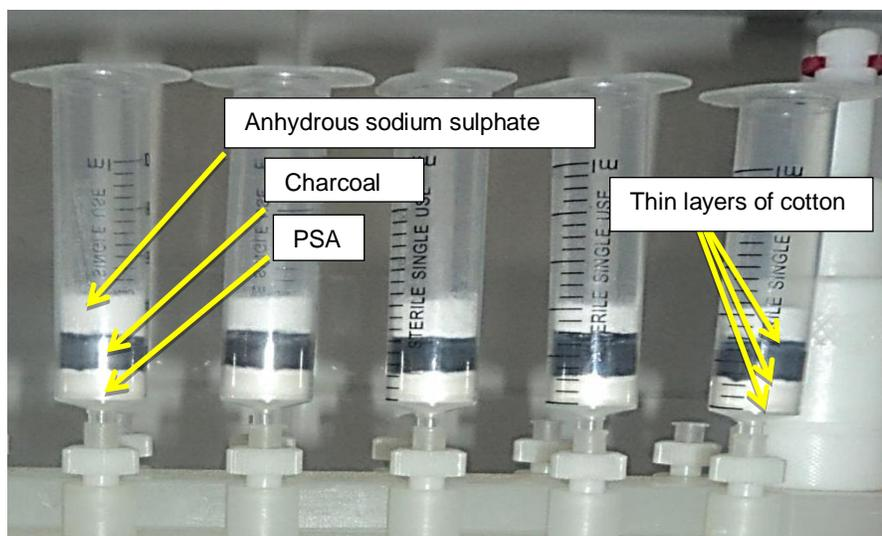
**Photo 2.** The Components of the Prepared Cleanup SPE Cartridges.
