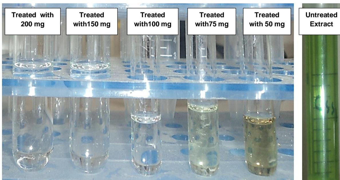
Photo 1. Effect of Charcoal Weights on Pigments Removal from Cucumber Sample Using d-SPE Cleanup. The Masses of Charcoal Varied from 50 mg/8 mL Extract to 200 mg/8 mL Extract.
